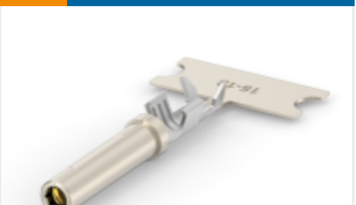
TE Part #1-2600021-5 XRC SOCKET 16-18 AWG Gold Plated
