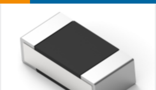
TE Part #8-2176307-5 RP 1E 0.1W 93K1 0.1% 25PPM 5K RL
